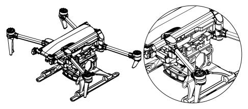
6. Move the EXOLANDER + EXOLock Mount back and forth on drone, confirming fit is locked into position.
