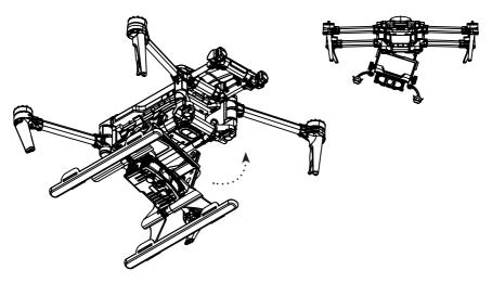
4. Pivot EXOLANDER so it is aligned straight with the drone base.
