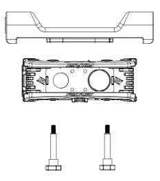
5. Adjust the tilt of the Rugo to desired angle and tighten the Mounting Knobs.
