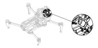
4. Confirm the Saddle is hooked properly to the drone and secured before flight by giving the saddle a slight jostle back and forth.
