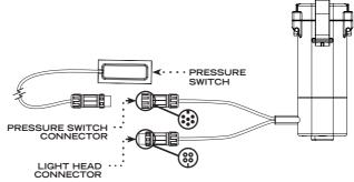
NOTE: # OF PINS AND MALE/FEMALE CONNECTOR ORIENTATION MAY VARY BETWEEN PART NUMBERS
