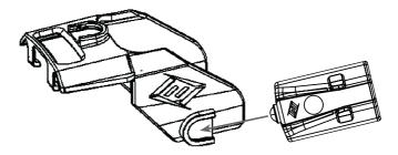
2 Take the Saddle with lights installed, and mount on the ANAFI USA, as shown below (lights are removed for simplicity).
