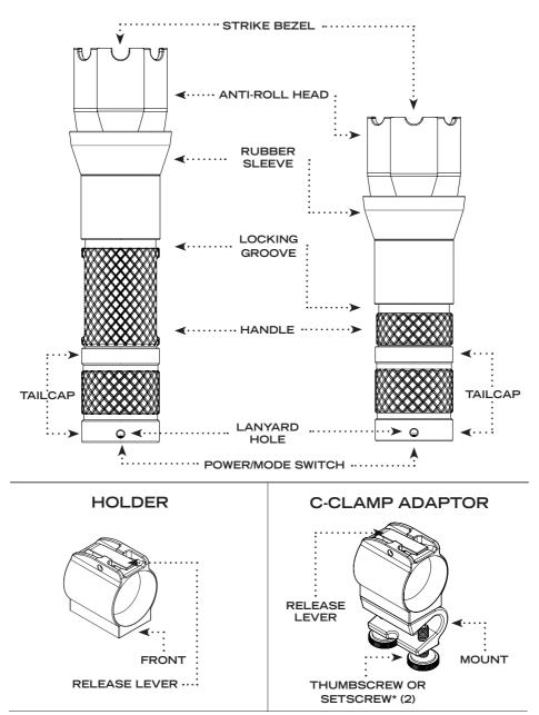
\*Newer model SideSlide C-Clamp and C-Clamp Mini comes with Setscrews instead of Thumbscrews.
