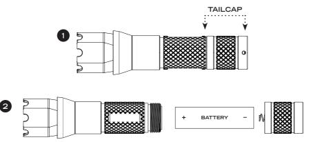
1 Twist the Tailcap in a counter-clockwise direction to remove it.
