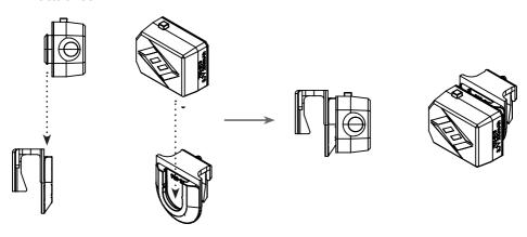
Take the mount with the light installed, and mount onto the DJI Avata, as shown below (lights are removed for simplicity).
