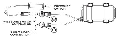
NOTE: # OF PINS AND MALE/FEMALE CONNECTOR ORIENTATION MAY VARY BETWEEN PART NUMBERS
