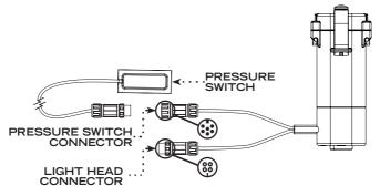
To connect the Pressure Switch Connector to the Pressure Switch, simply confirm alignment, insert the connector, and tighten the Screw Cap.
