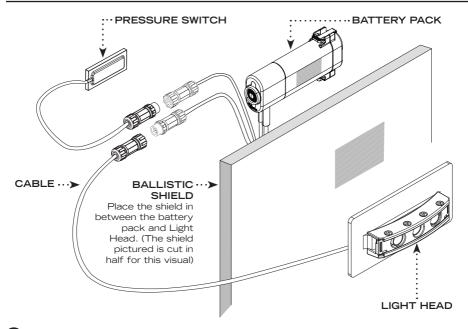
1 Clean the surface of the shield where the Battery Pack and Light Head will be placed.
