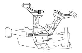
4. Align Locking Knob & Screw and Thread Locking Nut Insert on each side.
