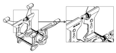
5. Tighten each screw until the units are mated.
