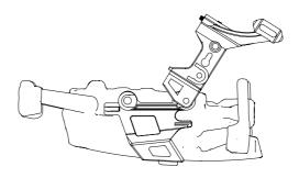
3. Install the other EXOLANDER® Half in the open Saddle Snap Lock locations. Bring the units together and align the Pin into the Hole on each side.
