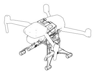
7. To install the Landing Skid, align each Tab on Landing Skid with each Slot on the EXOLANDER® Landing Foot. Press and snap Landing Skid on.
