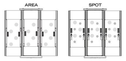
NOTE: The Sliding Diffuser Lens can be removed and cleaned for maintenance. Please reference p. 15.
