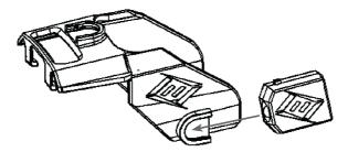
2 Take the Saddle with lights installed, and mount on the ANAFI, as shown below (lights are removed for simplicity).
