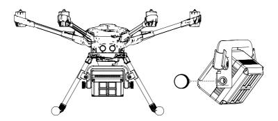
3. Tilt D100<sup>©</sup> to easily access the Switch and turn it ON to desired mode, and turn it ON to the desired mode.
