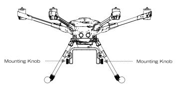
2. Align the Mounting Knobs with the  $^{1\!/\!4}$ -20 threaded screw holes on D100° to install D100° on the bracket.
