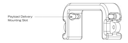
2. Align the Cross Bar on the larger hole of the Payload Delivery Mounting Slot and slide the crossbar into the locked position of the smaller slot hole.
