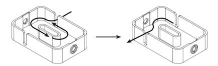
3. Use finger to keep the cable held in position around the Cable Retainer Boss. Press the Cover to the Base so that the Release Tabs align with the Release Tab Holes. Make sure that the Tabs are locked in the Holes.
