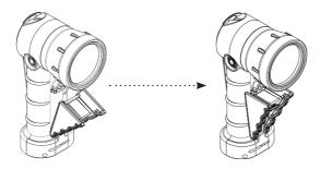
Place the narrow end of the Wedge on the bottom notch (located above the Battery Door). Maneuver the wide end of the Wedge to the top notch (located below the Charge Indicator).
