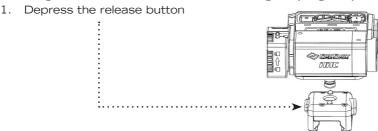
2. While holding the release button, align the coupling adaptor with the opening in the mount and insert.
