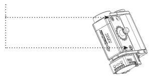
2. Attach the Molle Mount, with respect to HHC positioning in picture. Insert screws in appropriate holes then torque down with screw driver. Ensure to switch from counter sunk screws to the button screws provided.
