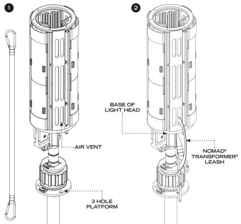
Begin with the Light Head installed on the Tripo-Scope® Pole or on the optional Nomad® Transformer® Extension. Make sure to have the Light Head at a reachable level so that the Transformer® Leash can be installed.
