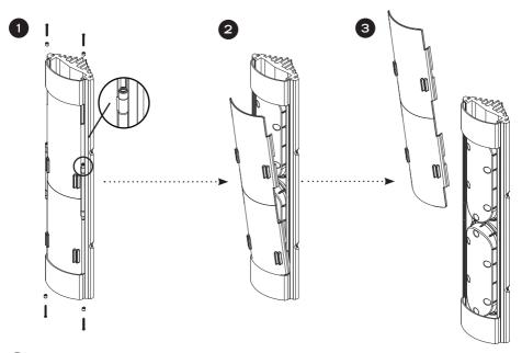
1 Slide the Sliding Diffuser Lens back into the 'Area' setting (see "Light Head Configuration" on p. 9). Find and remove the four (4) screws located on each side of it.
