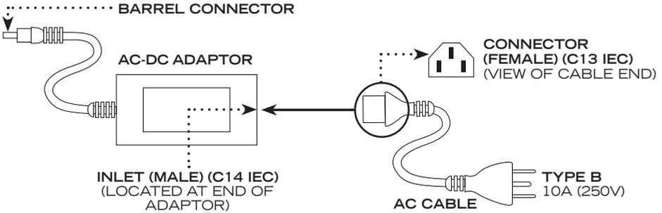
The plug of the AC Cable should be country specific. Example: IEC Types A-N. The Female Connector side of the AC Cable must be IEC Type C13 to mate with the Male Inlet of the AC-DC Adaptor.
