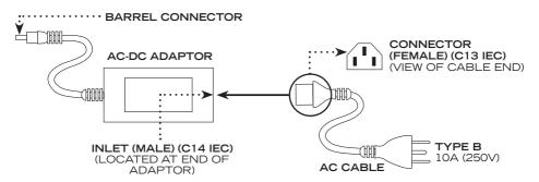
The plug of the AC Cable should be country specific. Example: IEC Types A-N. The Female Connector side of the AC Cable must be IEC Type C13 to mate with the Male Inlet of the AC-DC Adaptor.
