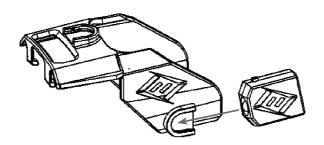
2 Take the Saddle with lights installed, and mount on the ANAFI, as shown below (lights are removed for simplicity).
