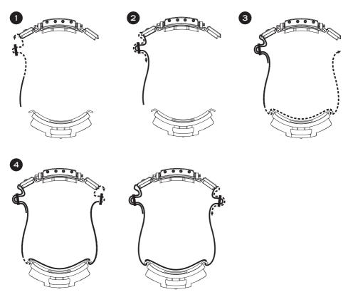
Place the headlamp on a flat surface. Position the Light Head so the Power/ Mode Switch is on the left and the LEDs face forward. NOTE: Make sure the FoxFury logo on the Battery Pack is correctly oriented before beginning.
