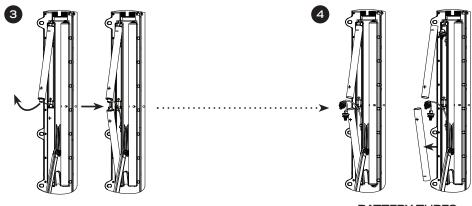
BATTERY TUBES REMOVED
