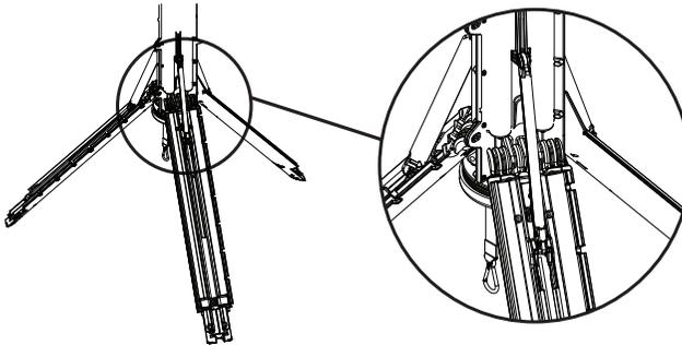
NOTE: The Anchor Strap retracts automatically, DO NOT let it retract back into the Tripo-Scope® M1 body without a D-Ring or Carabiner attached to it.
